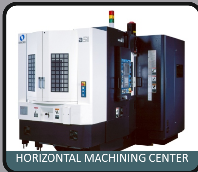
HORIZONTAL MACHINING CENTER
